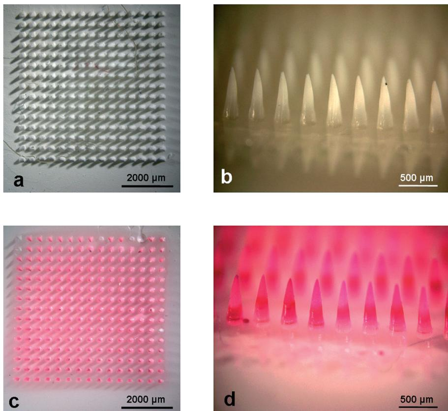
**Figure 1.** PVP polymer microneedles made by a new in situ polymerization process. a) Overhead view and b) side view of pure PVP microneedles. c) Overhead view and d) side view of PVP polymer microneedles with sulforhodamine encapsulated within microneedles and not within the base substrate. Each microneedle measures 750  $\mu\text{m}$  in height, 250  $\mu\text{m}$  in base diameter, and 5  $\mu\text{m}$  in tip radius.
