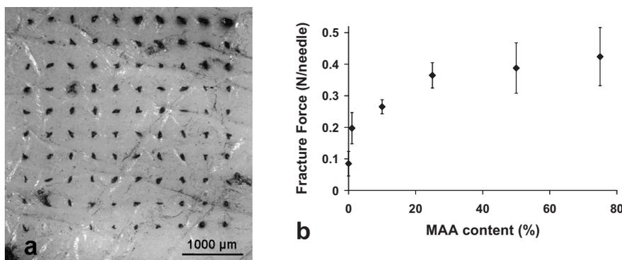
**Figure 2.** Insertion capabilities and mechanical properties of polymer microneedles. a) Evidence of insertion of PVP polymer microneedles into porcine cadaver skin via skin marking test. b) Plot showing the mechanical strength (fracture force) of the copolymer PVP-MAA microneedles increasing with increasing methacrylic acid (MAA) content.
